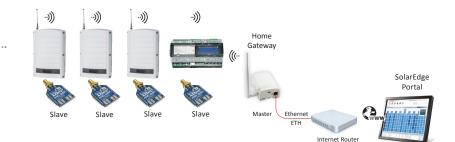
Example 3 ZigBee Wireless Server Connection
